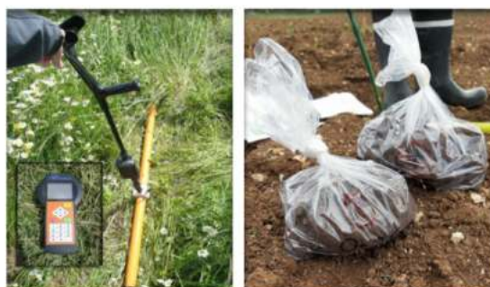
Figure 1. Apparent electrical conductivity (ECa) measurements using CMD Mini Explorer (left) and soil sampling (right)
