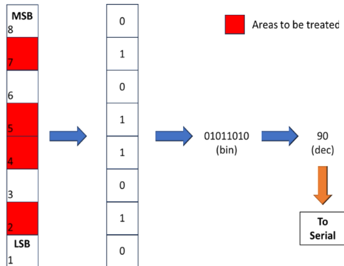
Figure 118. Summary of the procedure for converting the prescription map for each individual actuator into a single byte that can be sent via serial to the slave.
