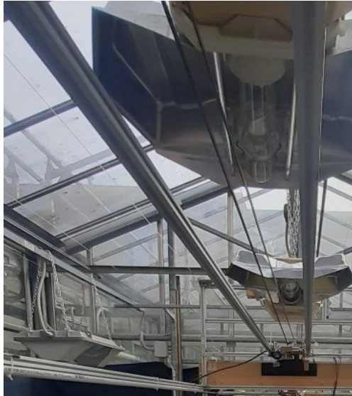
Figure 73. Overview of the linear actuator with the sensor attached underneath on the moving platform. The two rails and the drive belt are visible.
