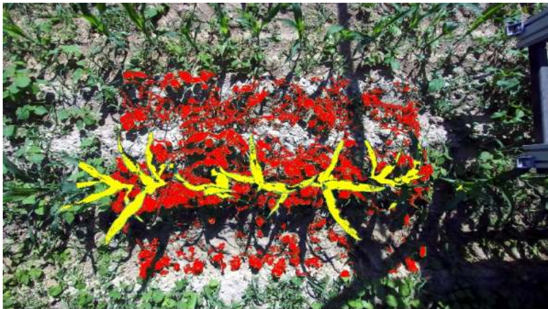
Figure 99. Example of binary crop-weed segmentation. An overlay is shown highlighting pixels classified as crop in yellow and those classified as weeds in red. The highlighted area corresponds to the workspace of 1 m x 1.5 m.
